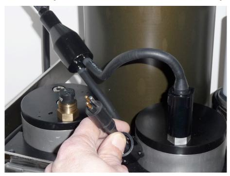
This connector is "live" with the voltage from the first battery pack. Plug it into the second pack immediately to reduce the risk of short circuits.
